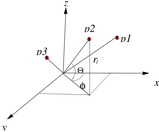
The application program moves a three-axis motion system from  $p1$  to  $p2$  and  $p3$  in the polar coordinate. The three points,  $p1$ ,  $p2$  and  $p3$  are characterized by their  $r$ ,  $\Theta$  and  $\phi$  as follows:
