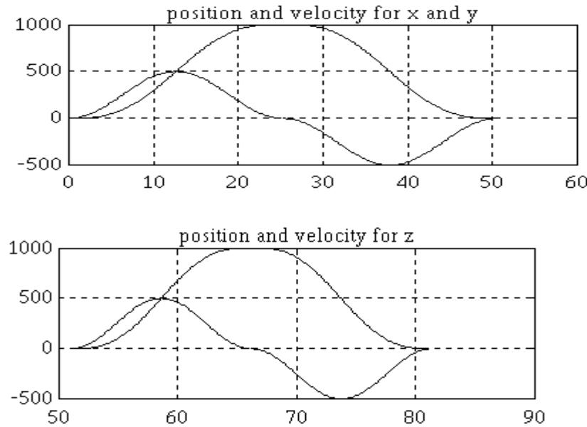
In the first example, axes x and y reach their targets simultaneously. The z axis starts its move upon the completion of x and y motion. We've separated z trajectory from x and y to point out that z can have its own independent shape.
